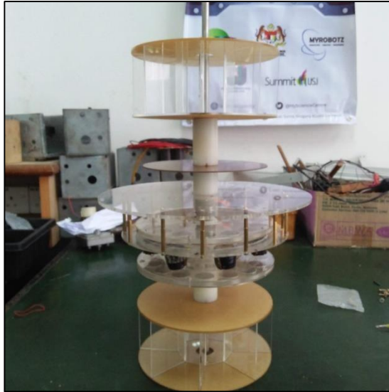
Figure 3.8: The axial generator for pico-hydro power generator while doing the process balancing and alignment.
