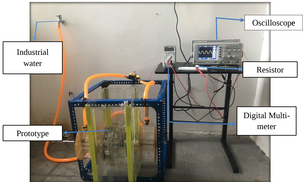
Figure 3.10: Experimental setup of the Double Rotational Axial Generator for Pico-Hydro Power Generation.
