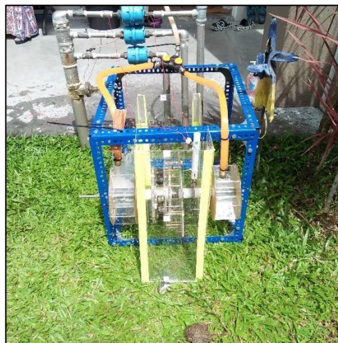
Figure 3.9: An axial generator for pico-hydro power generator successfully implemented.
